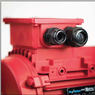
A large, square, cast aluminium T-box has been designed to meet NEC space requirements. Equipped with NPT and PG plugs, it can be rotated in 90 degree increments and boasts a wiring diagram embossed on to the back of the cover. There are no plastic cost outs here! Inside are clearly marked, stud type terminal blocks and leads marked in the proper IEC format.
